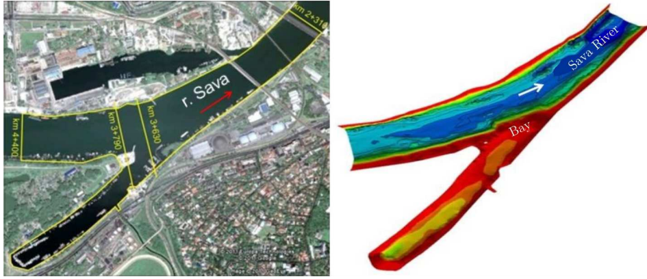
Figure 1: Computational domain and bathymetry; the Bay bottom is 8 m above the Sava River thalweg [6].
