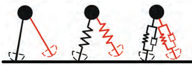
Figure 8. Bipedal walking models: inverted pendulum, spring mass and spring mass with damper, respectively. Solid lines represent each model in its basic, point-foot, mode, while the dashed line represent addition of rocker-foot
