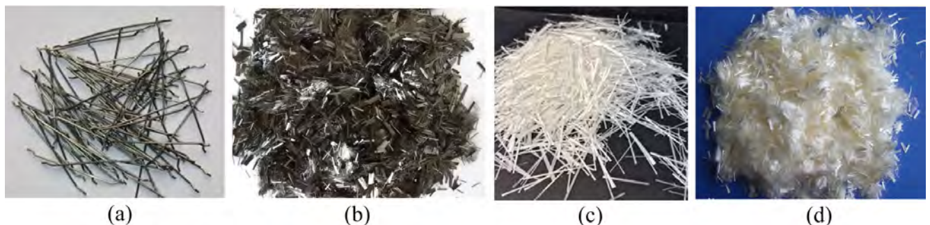
Figure 7. Types of fibres in FRC: a) steel, b) carbon, c) glass and d) polypropylene fibres
