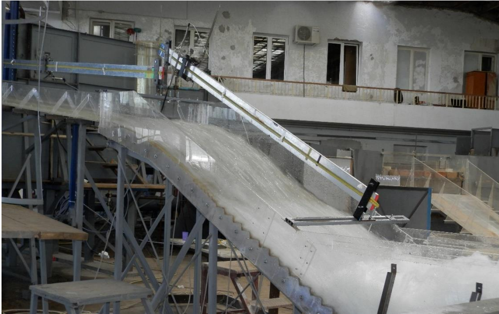
Slika 2. Model složenog brzotoka u razmeri 1:20. Figure 2. Scale model of complex chute, scale 1:20.
