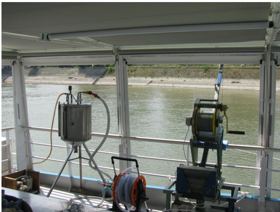
Figure 6. Equipment for the collection of water-column and bed samples
