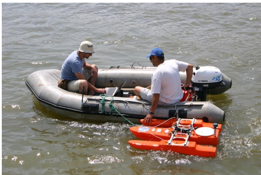
Figure 5. The flow discharge and velocity measurements equipment
