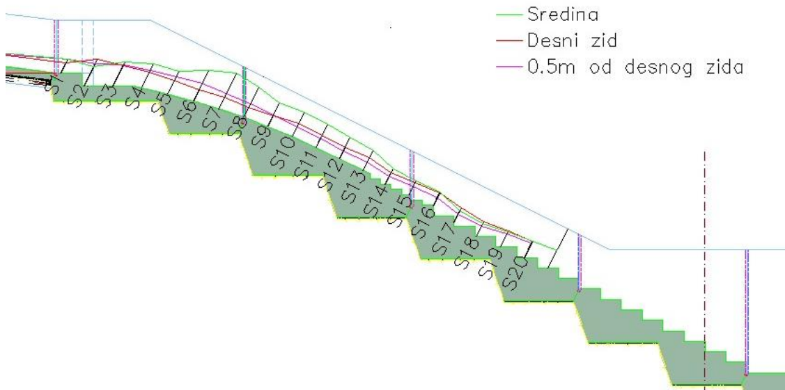
Slika 8. Linija nivoa na stepenastom brzotoku pri Q_{0.1\%}=236 \text{ m}^3/\text{s} i V_{ul}=18\text{m/s} za varijantu I. Figure 8. Water levels in stepped section of chute at Q_{0.1\%}=236 \text{ m}^3/\text{s} and V_{ul}=18\text{m/s} , alternative I.
