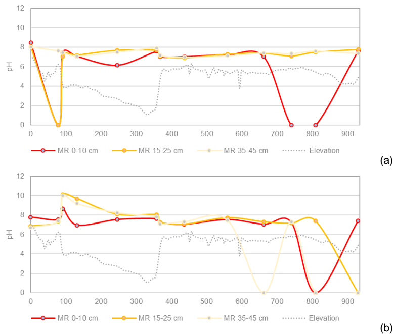
Figure 8. Change of pH measurements over the distance and elevation along the Pathway I during sampling event on: (a) 12/07/2018; (b) 31/08/2018. Zero values are the missing measurements.
