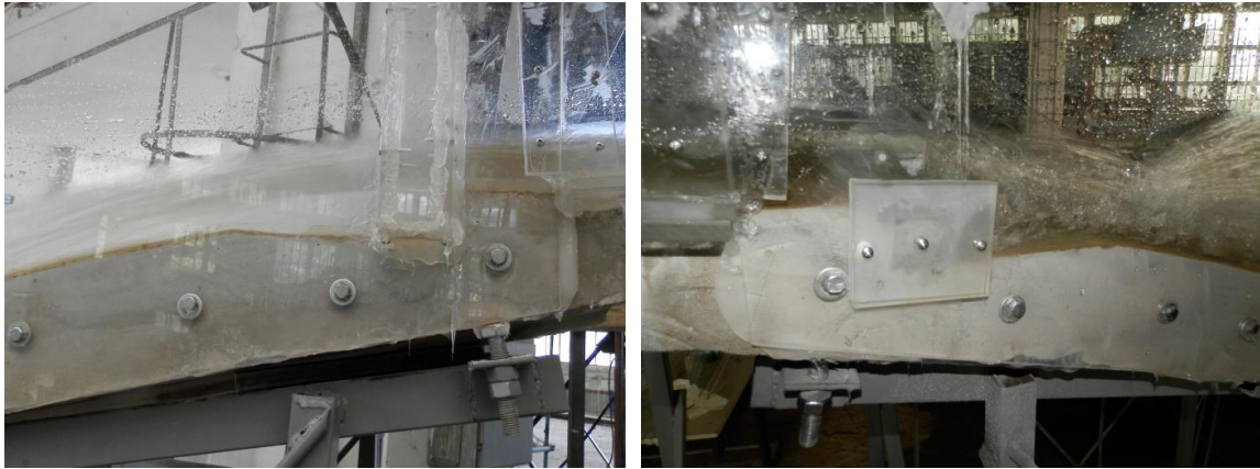
Slika 6. Mesto promene nagiba brzotoka za varijantu I (levo) i II (desno) pri Q_{0,1\%}=236 \text{ m}^3/\text{s} . Figure 6. The profile of slope change for alternative I (left) and alternative II (right) at Q_{0,1\%}=236 \text{ m}^3/\text{s} .
