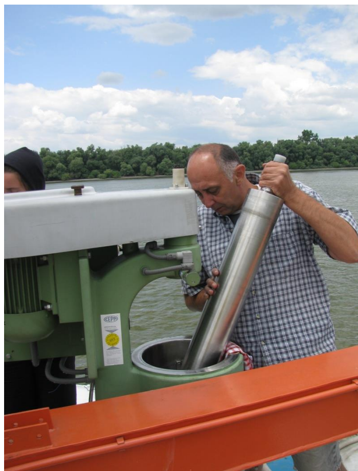
Figure 9. Equipment for the collection of suspended-sediment-quality analysis samples
