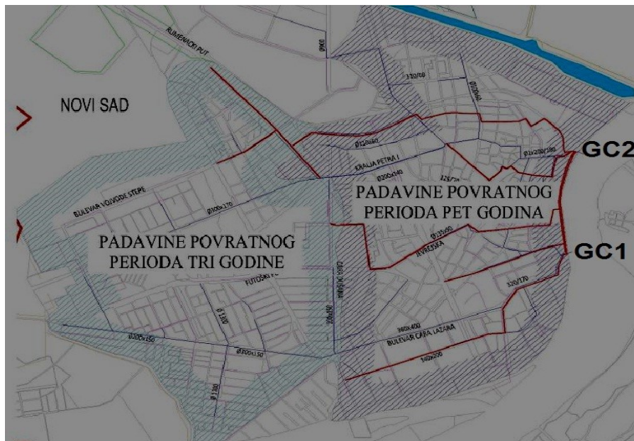
Slika 4. Raspedela kiša povratnog perioda od 3 i 5 godina Figure 4. Three- and five-year storms design for city area
