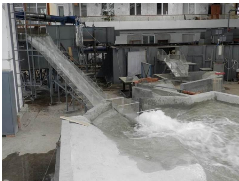
Slika 3. Model celine u razmeri 1:30. Figure 3. Complete scale model of labyrinth spillway, chute and stilling basin, scale 1:30.
