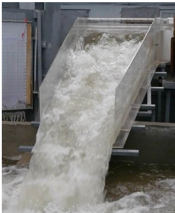
Slika 2. Polovina lavirint preлива i brzotoka na parcijalnom modelu, u razmeri 1:15 Figure 2. Half of labyrinth spillway and chute, partial scale model, scale 1:15.
