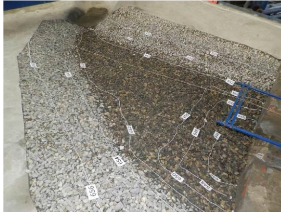
Figure 21. Erozija nizvodno od slapišta pri Q_{0.1\%} , projektovana nizvodna zaštita. Figure 21. Erosion downstream from the stilling basin at Q_{0.1\%} , including designed downstream protection.
