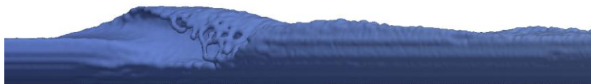
Slika 7. Izgled fluidne struje u krivini dobijen upotrebom SPH metode Figure 7. Location of the section where the wave reaches the pipe invert (side view)
