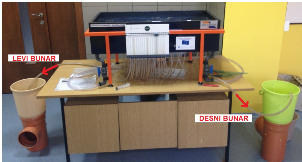
Slika 12. Laboratorijski model bunara Figure 12. Groundwater flow and well abstraction
