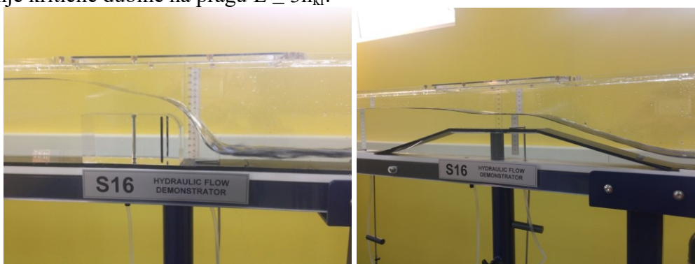
Slika 8. Oštrovični i zaobljeni široki prag Figure 8. Broad crested weir – general and roof shaped type
