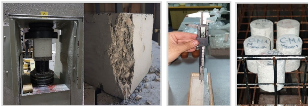
Figure 4. Compressive strength test (left), freeze/thaw surface resistance with a de-icing agent (middle), samples for freeze/thaw resistance (right)
