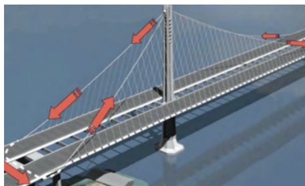
Figure 17. Diagram of load transfer on the Oakland Bay Bridge [12].
