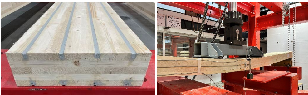
Figure 14. Hybrid FRP-CLT panel (left), static experimental setup (right)
