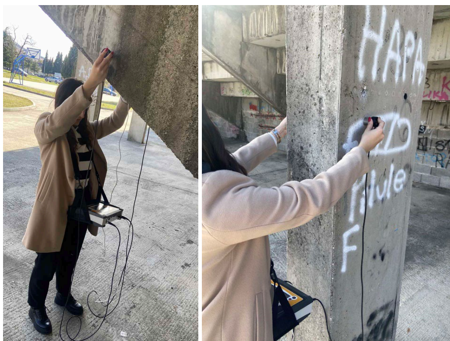
Figure 6. Ultrasonic pulse velocity test
