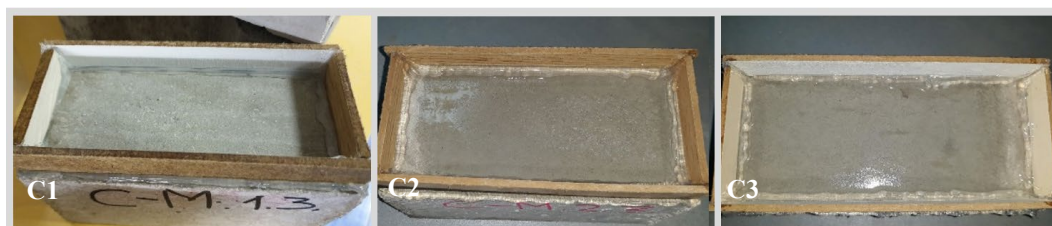
Figure 6. Surfaces appearance after 25 f/t cycles with de-icing salt
