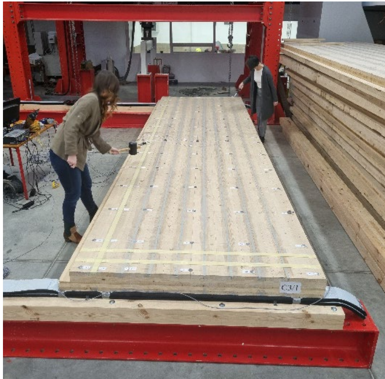
Figure 15. Modal testing of hybrid FRP-CLT panel
