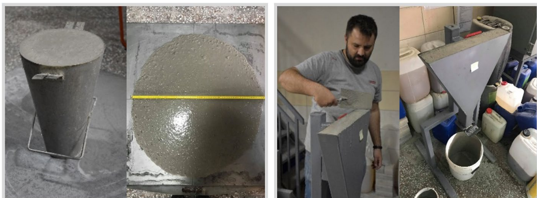
Figure 2. Flowability measurements using the slump-flow test (left), fresh concrete during V-funnel test (right)
