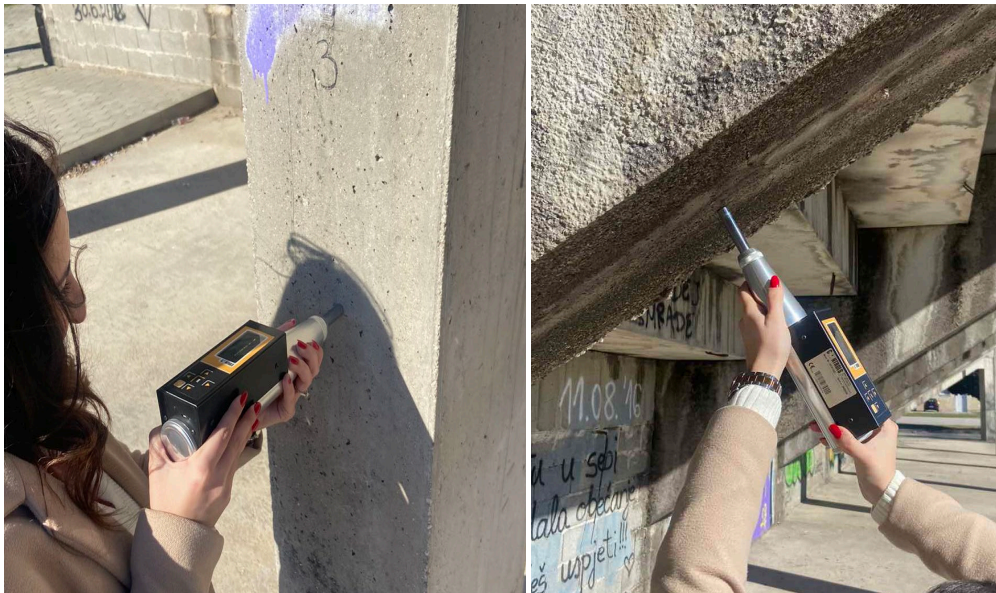
Figure 5. Compressive strength tests
