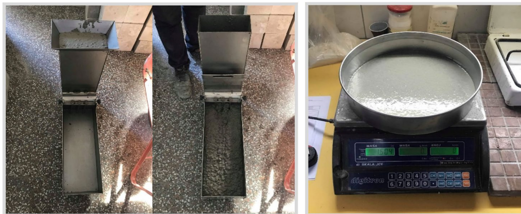
Figure 3. Passing ability testing, using the L-box (left), segregation resistance testing (right)
