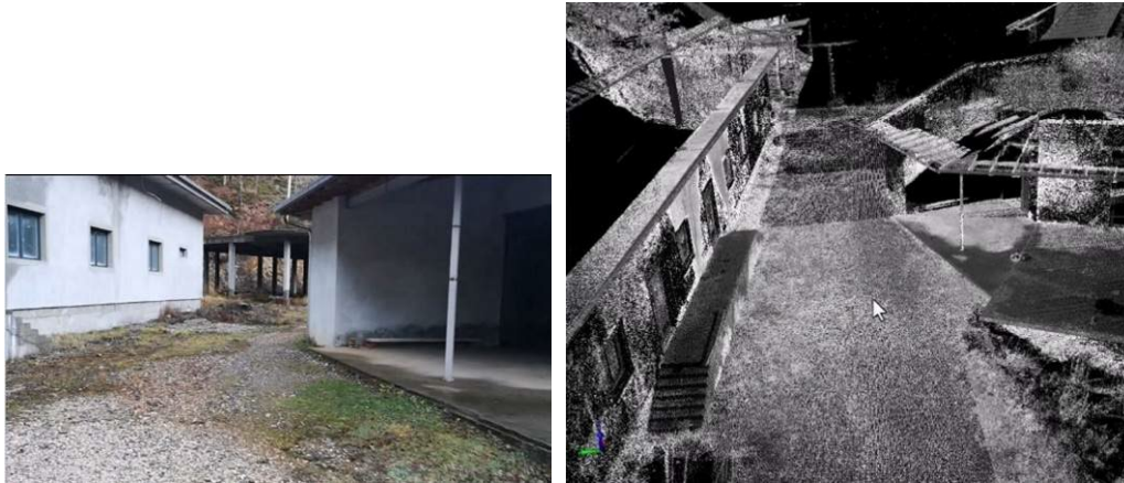
Figure 9. Actual situation (left), captured point cloud (right)
