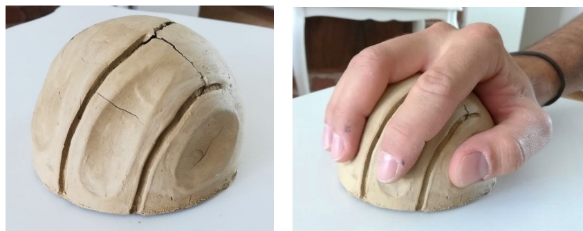
Figure 9: Clay model of the spherical element to determine optimal dimensions.
