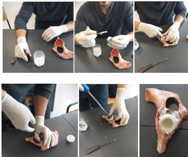
Figure. 10: Stages of attachment of the elements of the prosthesis using orthopedic cement
