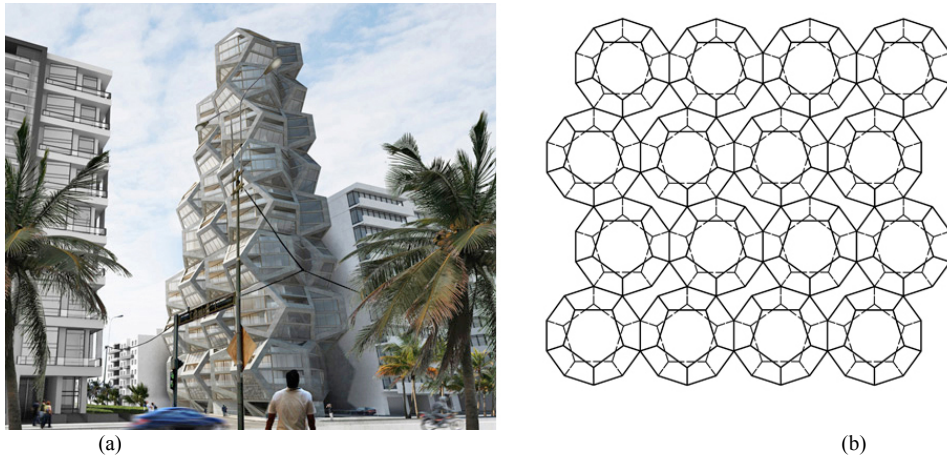
Figure. 7: (a) The Platonian Tower in Lima, Peru, and (b) Multiplication of The Dodecahedron (a) https://www.archdaily.com/500635/tammo-prinz-architects-propose-platonian-tower-in-lima 2014
