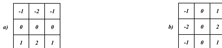
Figure. 5: 3-by-3 Sobel operator; a) derivative in y direction; b) derivative in x direction
