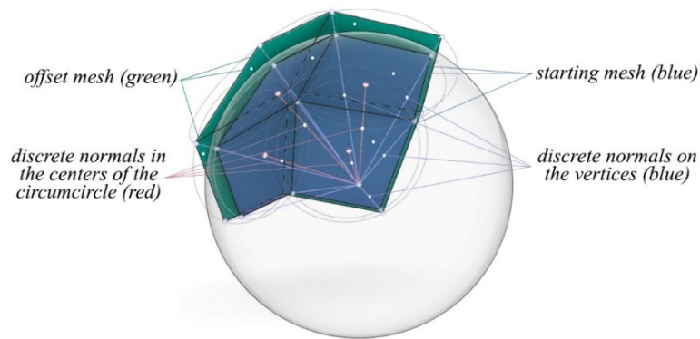
Figure 3: Display of two sets of discrete normals of the circular mesh system
