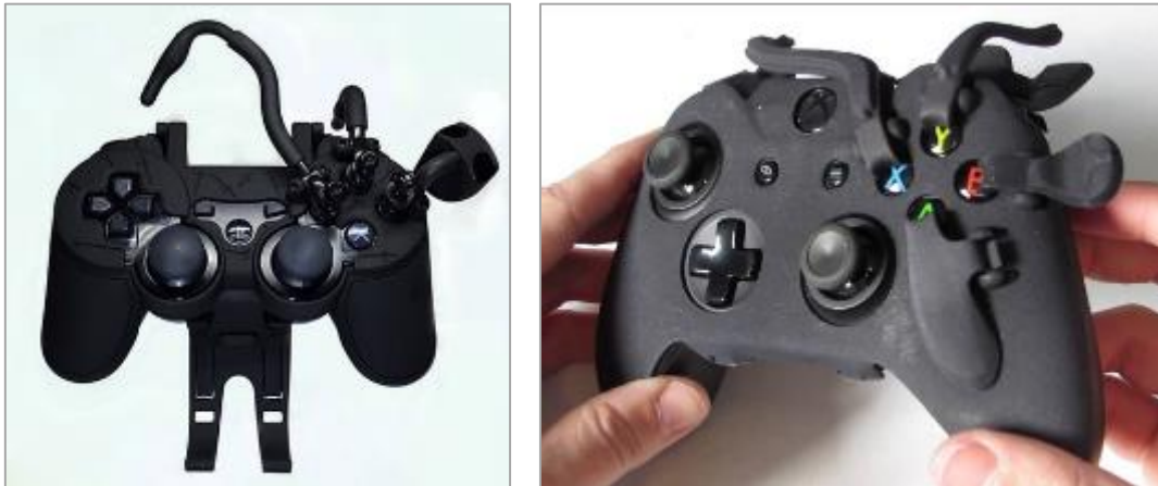
Figure 4: Modifications of standard controllers with custom made masks/elements. (Source: Maggiorini et al. 2019);
