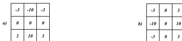
Figure. 6: 3-by-3 Scharr operator (OpenCV implementation); a) derivative in y direction; b) derivative in x direction
