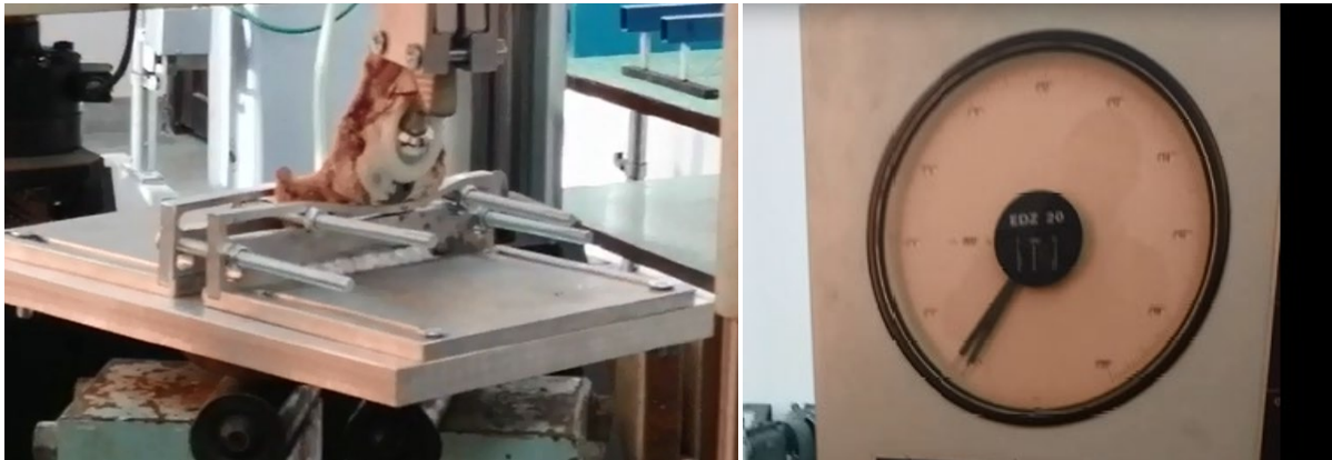
Figure. 13: The orthopedic system tested on the universal machine after failure
