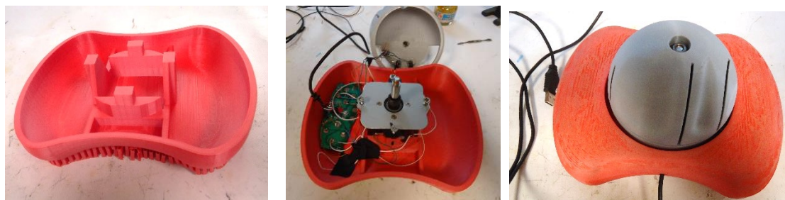
Figure 10: 3D printed model of the base, subassembly and the final prototype of the controller.
