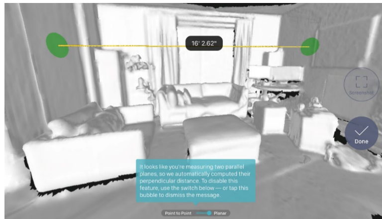
Figure. 4: AR space capturing using TOF camera (O'Kane, 2016)
