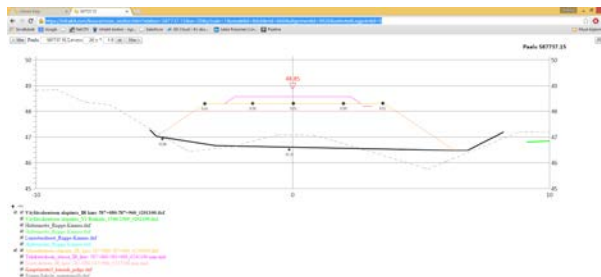
Figure 7. Cross section from position shown on image 6. Shows different layers and as-built points (red crosshairs and crosses) compared to design layers.
