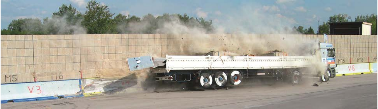
Figure 8. Crash test TB 81, 38t articulated lorry Source: Photograph © DELTA BLOC International GmbH
