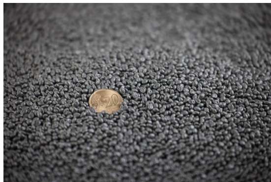
Figure 7. Example Polymeric Compound added directly in the mixer
