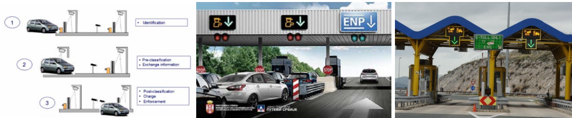
Figure 5. ETC DSRC with barriers tolling
