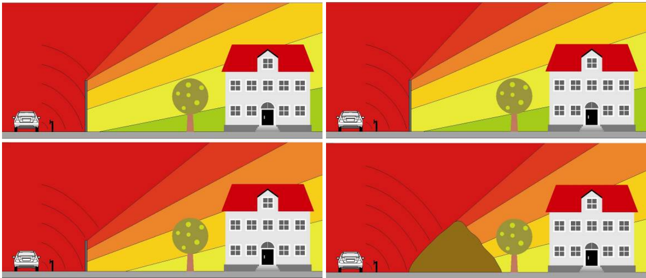
Figure 1. Comparison of noise dissipation with high (top) and lower (bottom) noise barriers Source: Graph by DELTA BLOC International GmbH
