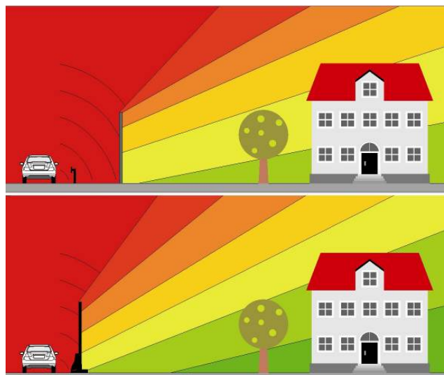
Figure 6. Comparing the noise dissipation of a standard noise barrier (top) and one with integrated vehicle restraint system (bottom) Source: Graph by DELTA BLOC International GmbH
