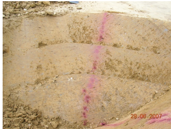
Figure 4. Indication of good homogeneity using phenolphthalein test.
