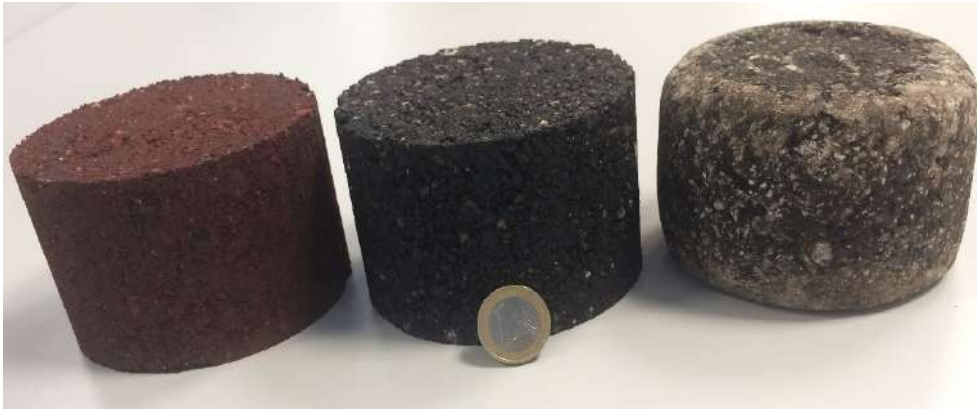
Figure 4. Marshall Compacted specimen compared with and without red coloring materials (sample) and before and after Cantabro test (scale coin 1€: 23.25 mm)
